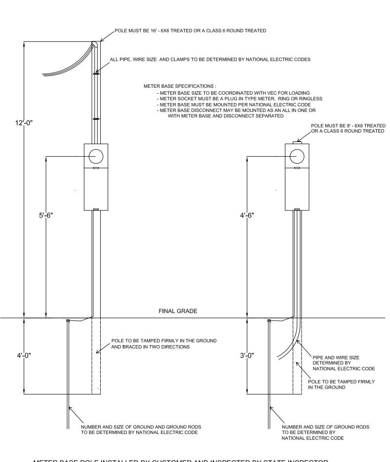
METER BASE POLE INSTALLED BY CUSTOMER AND INSPECTED BY STATE INSPECTOR
